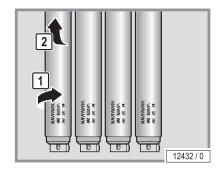
UV low pressure lamps possess a reflector which directs the light outwards. The lamps must be mounted in such a way that the rear side of the reflector is located on the device side.
