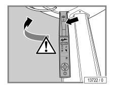
Carefully pull the panel past the back of the cockpit control and remove to the left.
