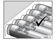
Push the pins vertically into the socket from above.
