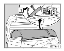
The canopy panel must be completely removed from the device in order to replace the lower, long UV low pressure lamps.
