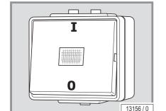
The electrical installation must have a freely accessible, all-pole disconnecting device (Master switch with clearly labelled On/Off settings, e.g. '0' and 'l' or additional indicator light) fitted externally on the side.
