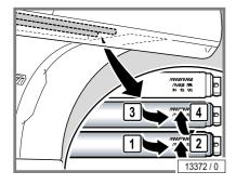
Remove the two upper low pressure lamps in the canopy so that you can then access the facial tanner's low pressure lamp starter.
