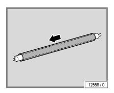
Slide the makrolon tube onto the new lamp.
