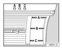
The facial tanner's low pressure lamps must be removed first so that the UV high pressure lamps and the filter panels can be changed.
